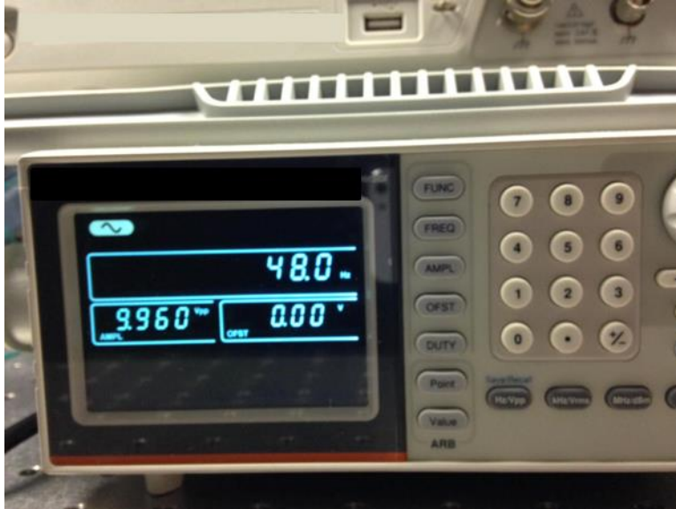
Figure 4.4: Use the FREQ button (second from the top, on the right next to the display panel) to adjust frequency.
