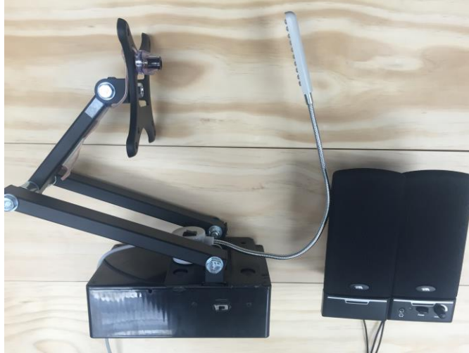
Figure 2.1: Depiction of the setup containing the photo resistor, lamp and speakers. The lamp faces the light sensor, which correlates light intensity with sound volume.
