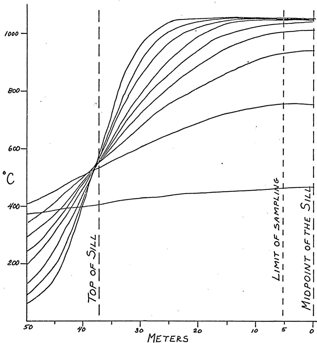
Figure 15. Theoretical cooling curve for Cedar Creek sill. Solid lines represent isotherms, dashed lines represent sill boundary and limit of sampling. Only half the sill is represented, the other (lower) half being theoretically symmetrical.
