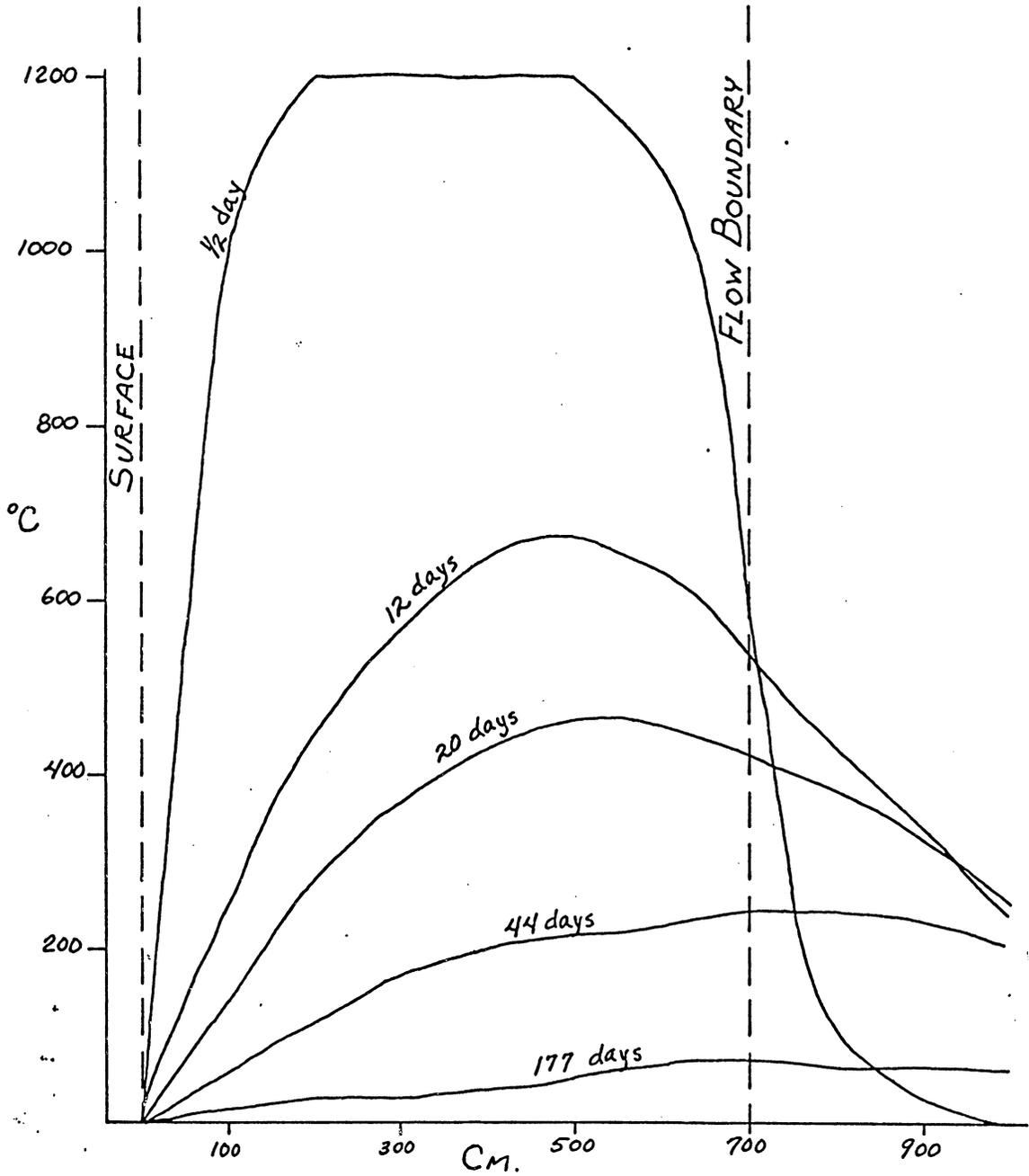
Figure 14. Theoretical cooling curve for the Mexico City flow. Dashed lines represent the flow boundaries, and solid lines isotherms at each time.
