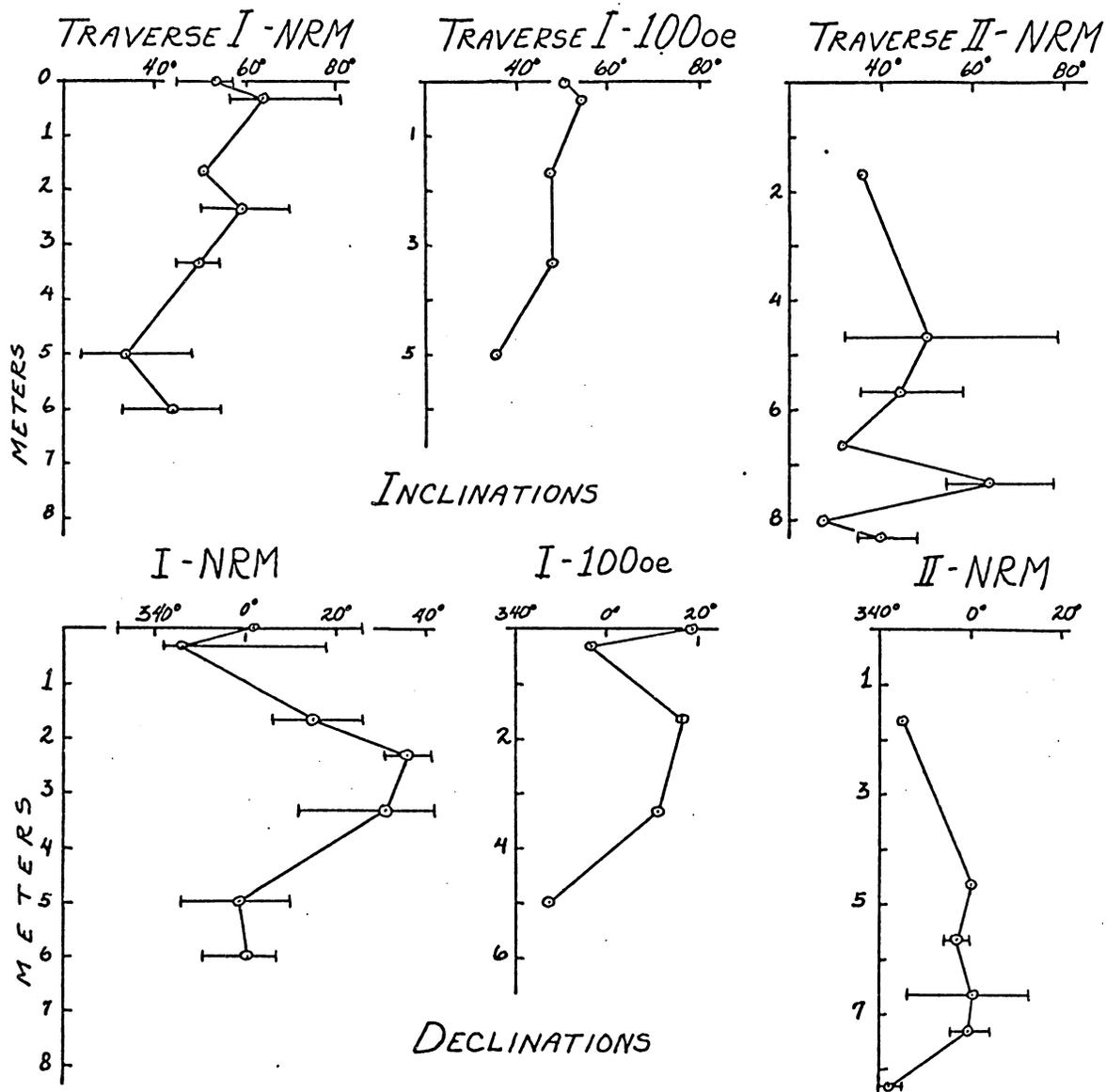
Figure 6. Inclination and declination versus position in the flow, traverse I and II, Mexico City. Bars on the original magnetization lines represent the range of values, points represent the averages.
