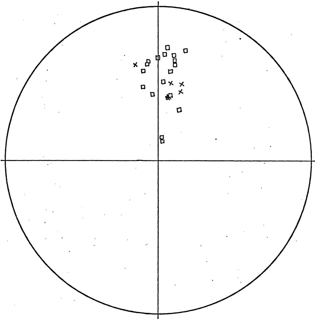
Figure 7. Demagnetized directions (100 oe) for traverse I (x), and original magnetization for traverse II ( $\square$ ), showing the rotation of the traverse I directions toward those of traverse II. Present field (\*).
