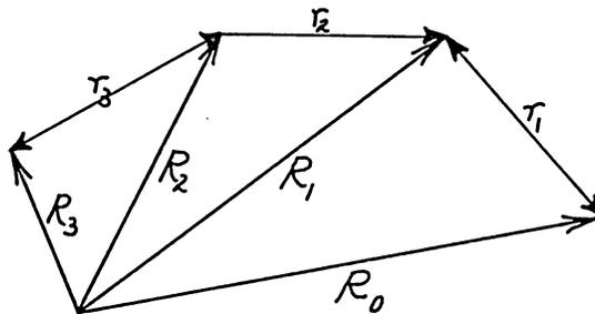
Figure 4. Vector representation of the stability number (S number) calculation.  $R_0$  is the original direction,  $R_1$ , after the first demagnetization, etc.;  $r_1 = R_0 - R_1$ . The non-vector sum of the  $r_i$ 's gives the r of the equation. The vector sum would be  $R_0 - R_i$ , which represents only the change from  $R_0$  to  $R_i$ , not the intermediate changes.
