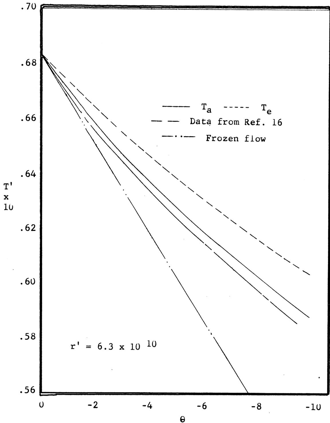
Temperature at a constant radial distance versus local flow deflection angle
