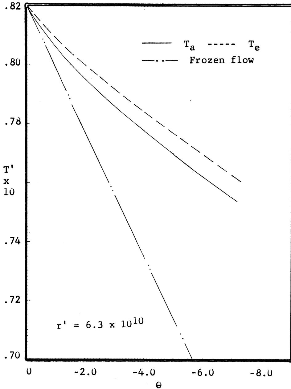
Temperature at a constant radial distance versus local flow deflection angle
