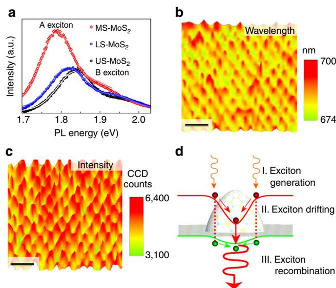
**Figure 3 | Scanning PL spectroscopy of the MoS<sub>2</sub> strain crystal.**
