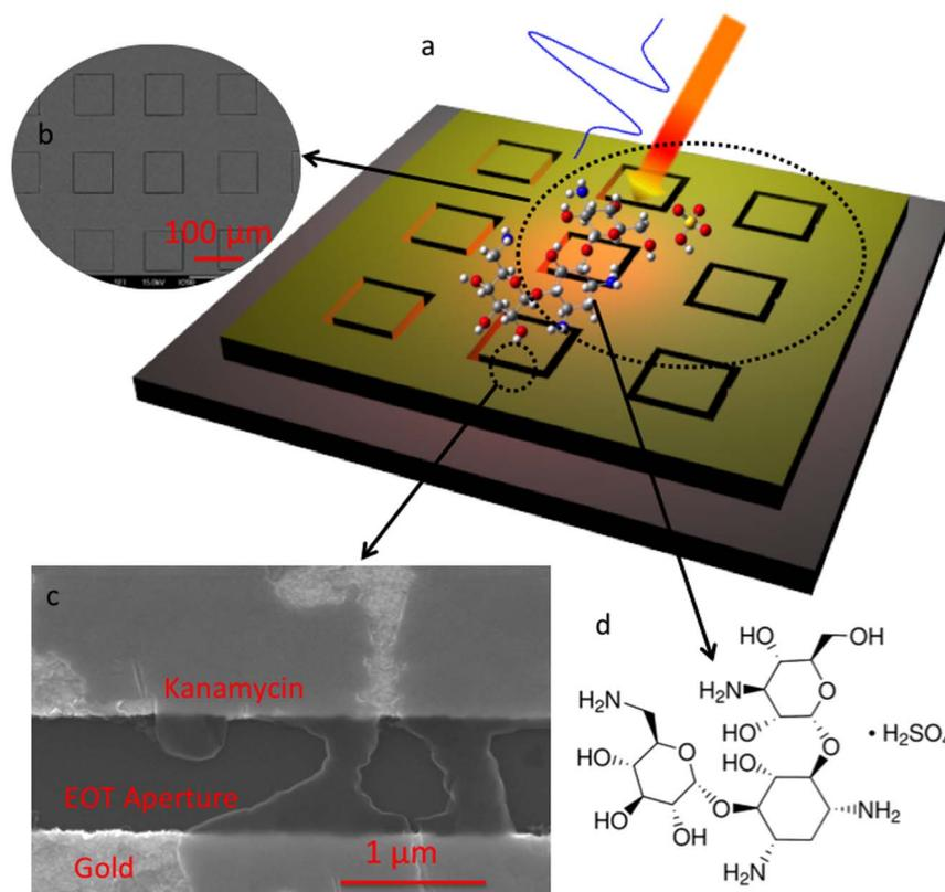
**Figure 1** | Metasurface-assisted THz sensing of kanamycin sulfate. (a), Schematic of the metasurface structure with kanamycin sulfate molecules deposited on the surface. (b) and (c), SEM images of the metasurface. (d), Kanamycin sulfate molecular structure.
