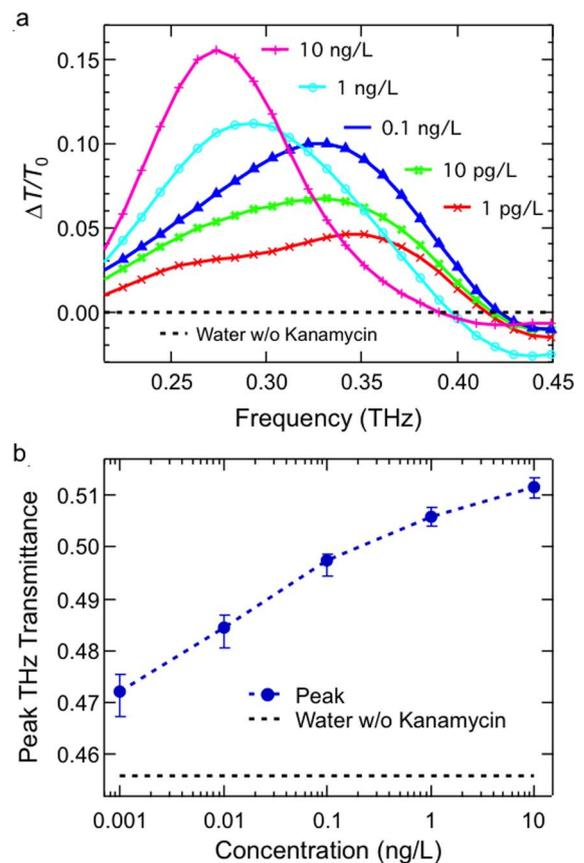
**Figure 3** | (a), Fractional change of transmittance versus frequency for kanamycin sulfate with 1 pg/L (red), 10 pg/L (green), 0.1 ng/L (blue), 1 ng/L (cyan), and 10 ng/L (pink) concentrations. (b), THz transmission peak value versus concentration.
