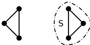
Figure 1.2 : Example of a violated subtour constraint that prohibits a solution containing subtours. The cut around the vertex set S (dashed line) is not crossed by at least 2 edges. Thus, it violates the constraint.
