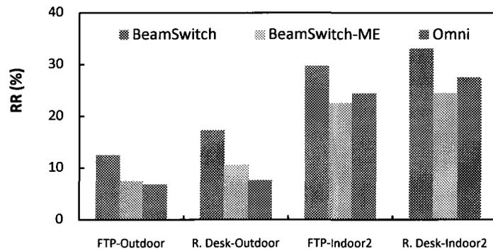
**Figure 11: Motion estimation (BeamSwitch-ME) reduces retransmission rates (RR) of BeamSwitch at 360°/s to very close to the conventional isotropic design**
