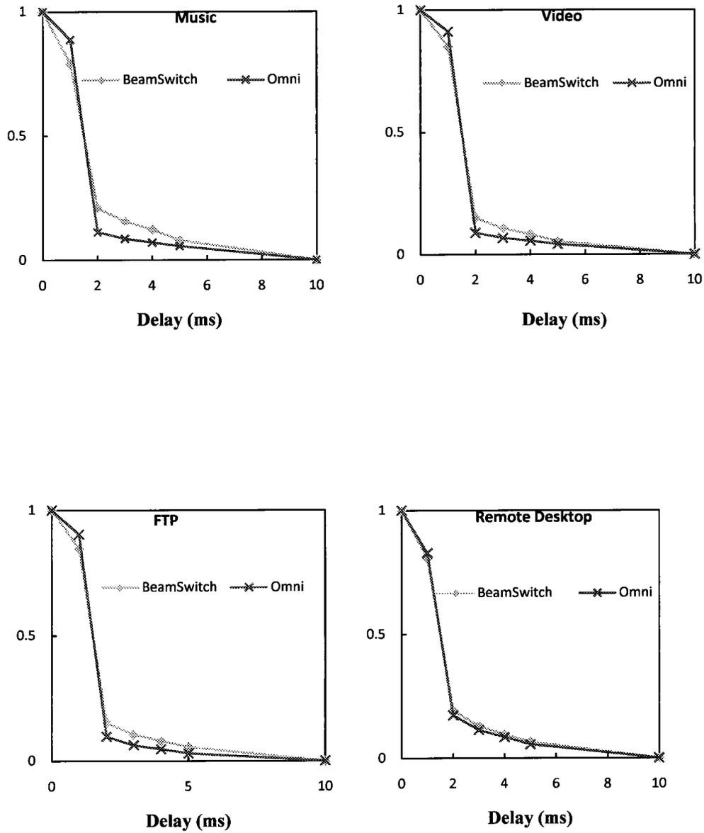
**Figure 7: Cumulative data delay distributions under *Indoor with People* as BeamSwitched node rotates at 360°/s**
