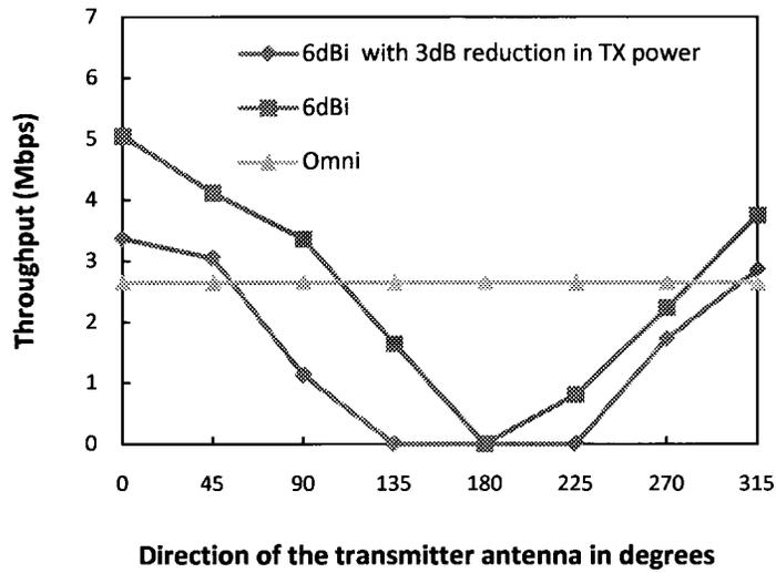
**Figure 2: FTP throughput between two wireless nodes as the node with a directional antenna (6dBi) changes its orientation from 0 to 315°**
