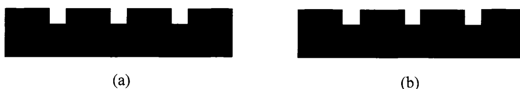
Figure 1.7 – The two allowed plasmon modes for a rectangular profile grating: (a) low energy anti-symmetric standing wave plasmon mode and (b) higher energy symmetric plasmon mode.
