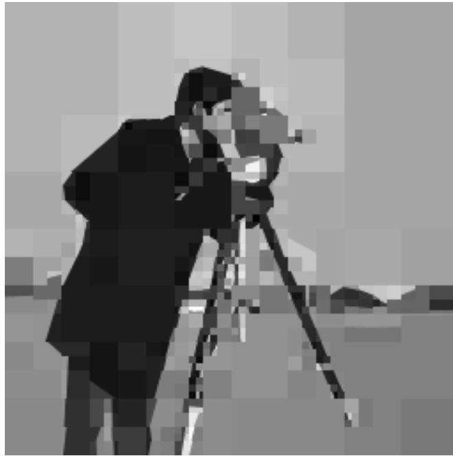
Figure 3.4 Cartoon sketch \bar{c} obtained from the coded wedgelet parameters, 0.12 bpp, PSNR = 22.28dB. Note the blocking artifacts at the wedgelet borders.
