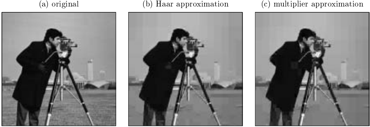
Figure 4. n -term approximation of the 256 \times 256 cameraman image ( n = 2103 ). The original cameraman image is shown in (a). (b) L_2 2103-term approximation using Haar coefficients, \|\hat{x} - x\|_2 = 581.8 . (c) KL 2103-term approximation using multipliers, d_{KL}(x, \hat{x}) = 57940.1 .
