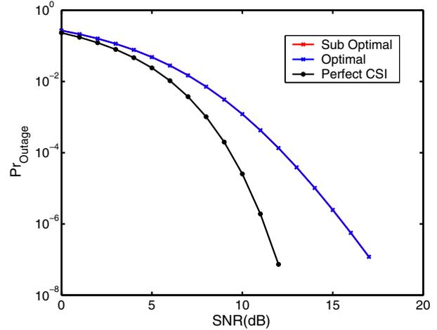
Fig. 2. Outage for  $\log_2(3)$  bits of feedback for optimal, equal allocation power control, and perfect CSIRT with respect to SNR for a system with single antenna at transmitter and receiver, and transmission rate of  $R=2$  b/s/Hz
