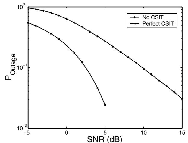
Fig. 1. Outage probability as a function of SNR with full and no channel state information at the transmitter (CSIT) for a single transmit-receive antenna system; receiver is assumed to have perfect channel information.
