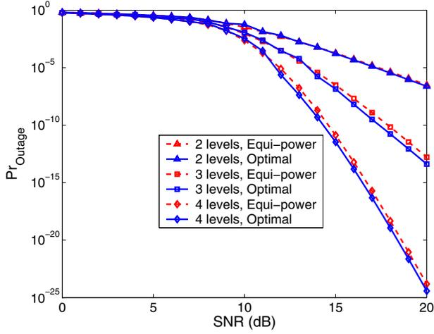
Fig. 3. Outage probability as a function of SNR for a system with 1,  $\log_2(3)$ , and 2 bits of feedback, 2 transmit antennas, and rate  $R=2$  bit/s/Hz.
