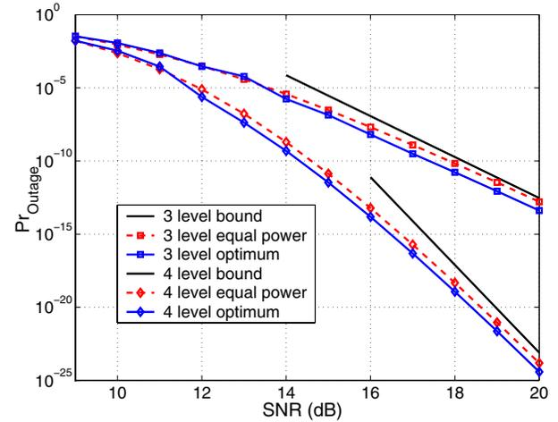
Fig. 4. Shows the bound on diversity order for  $L=3$ , and 4 with optimum and equal power allocation schemes for a system with 2 transmit antennas, and rate  $R=2$  bits/Hz.
