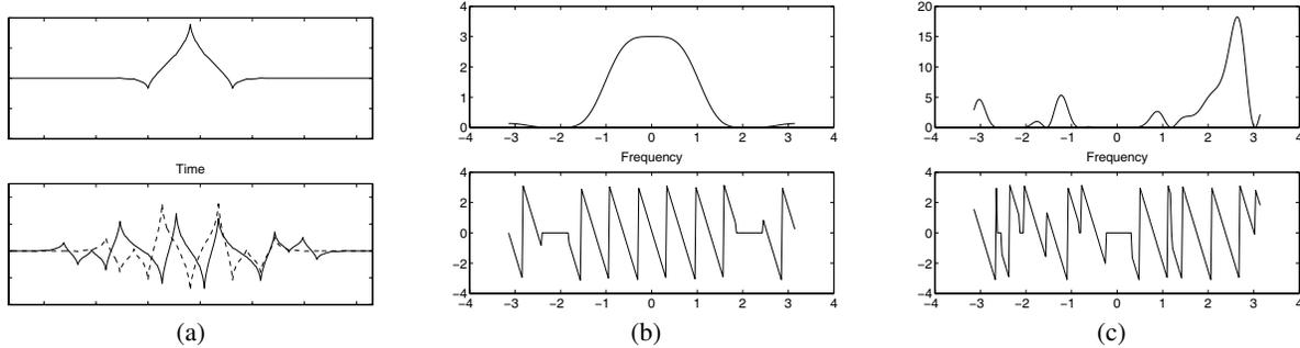
**Fig. 7.** (a) Top: scaling function associated with  $H_0(z)$ . Bottom: complex wavelet associated with  $H_+(z)$  (real part solid; imaginary part dashed). (b) Magnitude and phase response of  $H_0(z)$ . (c) Magnitude and phase response of  $H_+(z)$ .
