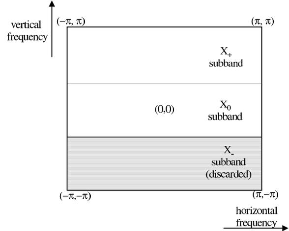
Fig. 5. Frequency-domain partitioning after 1D NCWTR on image rows.
