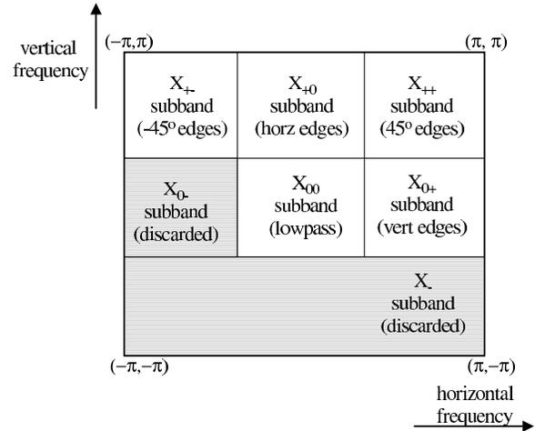
Fig. 6. Frequency-domain partitioning after 2D NCWT.
