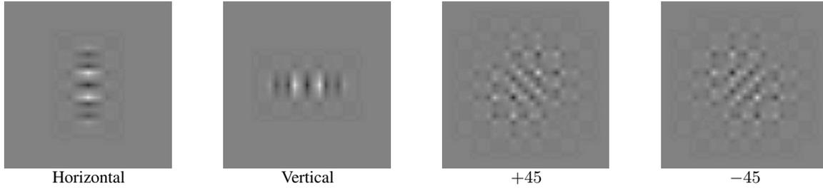
Fig. 8. 2D complex wavelet basis functions (imaginary parts shown).
