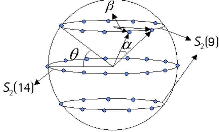
Fig. 1. A three-level three-dimensional real spherical constellation
