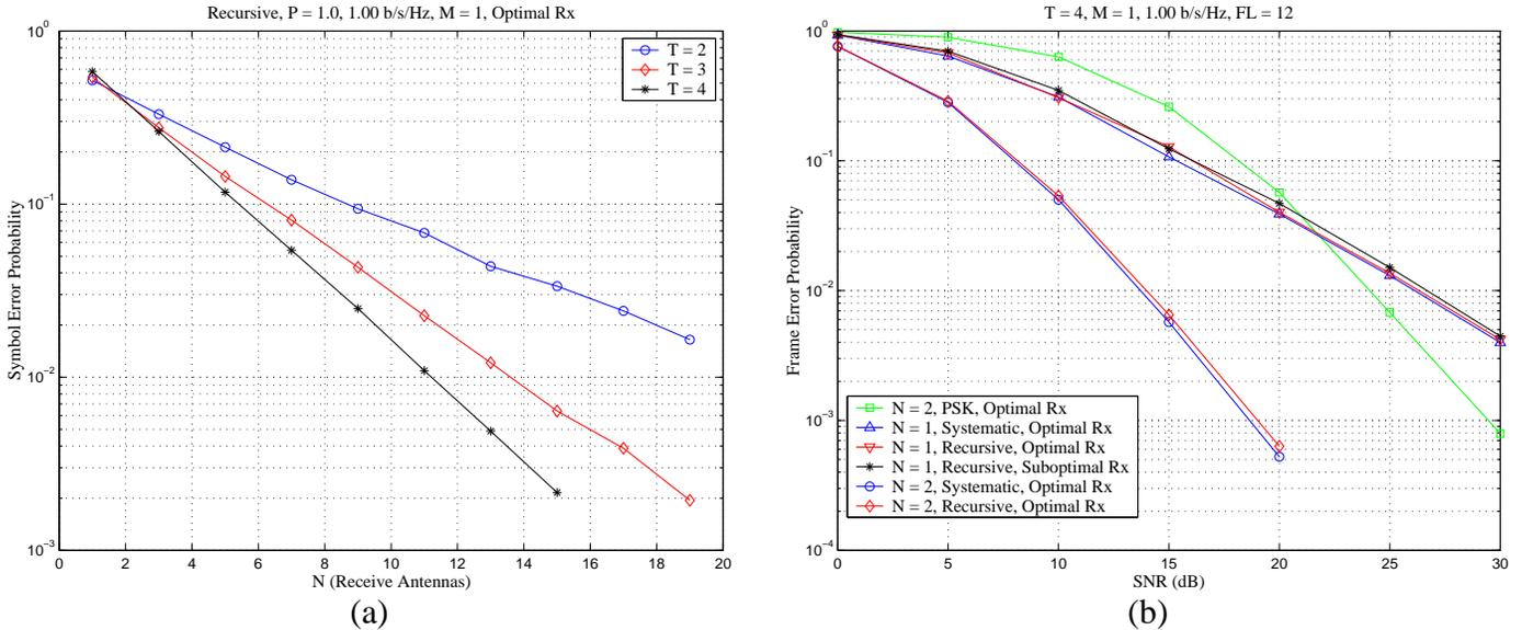
Fig. 4. Performance comparison of (a) recursive constellations with different values of  $T$  vs.  $N$  (receive antennas) at 0 dB, and (b) recursive constellations with systematic unitary constellations of [2] and PSK constellations of [3] for  $N = 1$  and 2, vs. SNR
