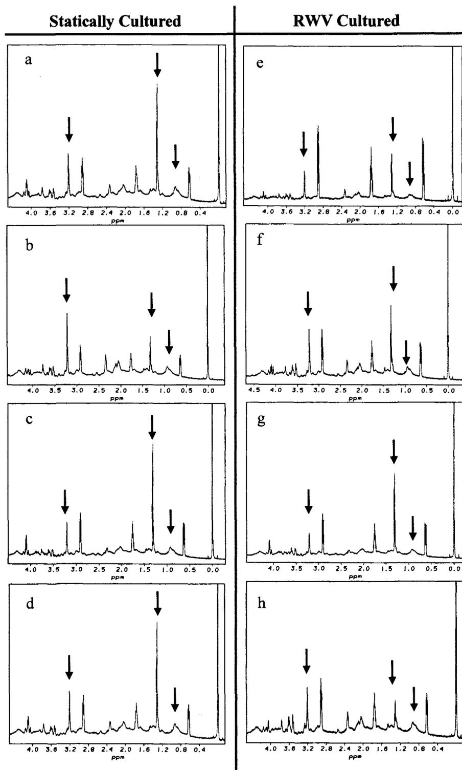
**Figure 3-4a-h: Time course study of Jurkat cells cultured under static and low shear conditions.** Arrows indicate peaks of interest:  $[N+(CH_3)_3]$ , 3.2 ppm; methylene  $[(CH_2)_n]$ , 1.3 ppm and methyl  $[CH_3]$ , 0.9 ppm.
